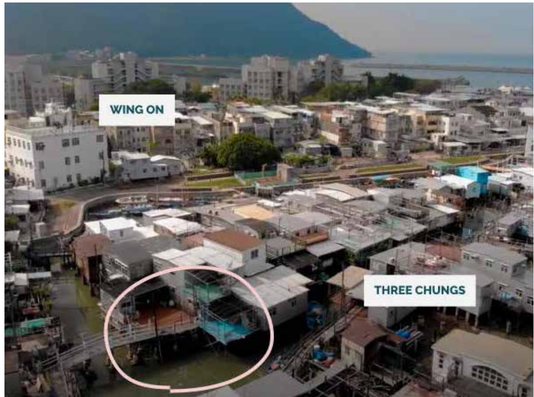
Aerial Shot of Wing On and Three Chungs, when Tai O is not hit by floods. Pink circled part demonstrates how the poles at the stilt houses are normally exposed in the air, instead of being immersed in water (taken by the research team)
